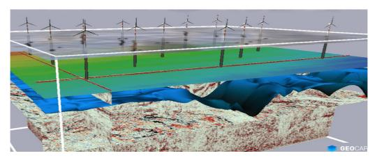
Offshore wind is fast becoming a major source of clean energy around the world and is projected to grow 10-fold from 2022 to 2050. All developments require a reliable and fit-for-purpose integrated ground model to help mitigate risks, design suitable anchor and/or foundation types and determine the most appropriate cable routes, burial and method for cable/foundation installation in a cost-effective and safe way.
